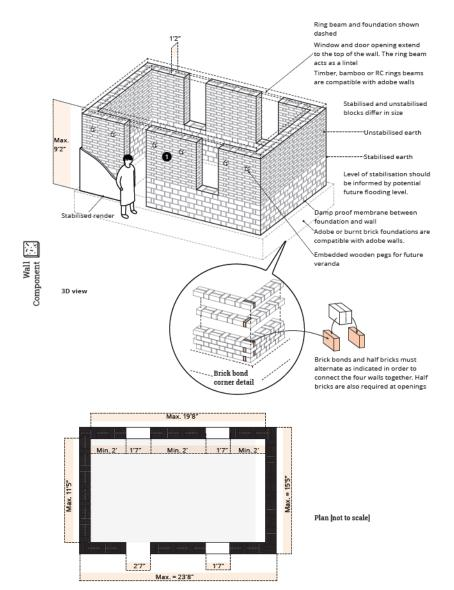
Seismic consideration: Sindh is a region of moderate to high seismicity. Seismic design is outside the scope of this guide, the following measures will improve seismic performance. The following is recommended: Remove front window; Use a reinforced concrete ring beam; Use piers at the corners and in the middle of the long wall. For more information see Design Information, Seismic page
