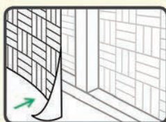
Double walls, for example using amakan, tarpaulin, or plywood on the inside of walls. This will provide better thermal and acoustic attenuation and increase privacy.
