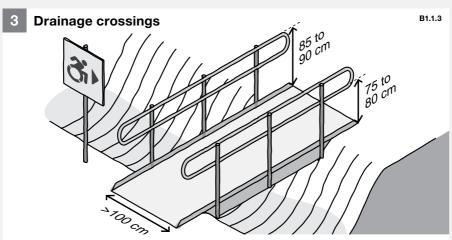
Surface water drainage should not create barriers for persons with disabilities. Open drainage canals need crossing points with signage and handrails for support. The design of these may vary.
