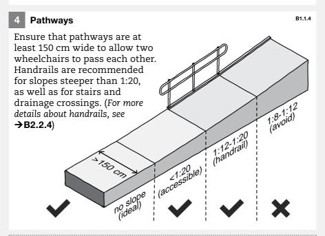
Compacted gravel or selfbinding aggregate is suitable as ground cover for pathways. Provide shaded resting places at 100-200 metre intervals along main circulation routes.
