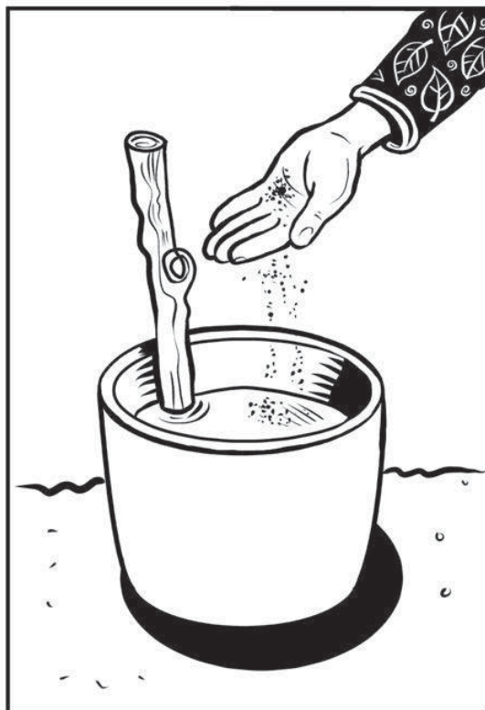
Fig 111: Add small amounts of earth pigments for colouring limewash. Mix well. (Mix enough quantity to cover an entire wall for colour match)
