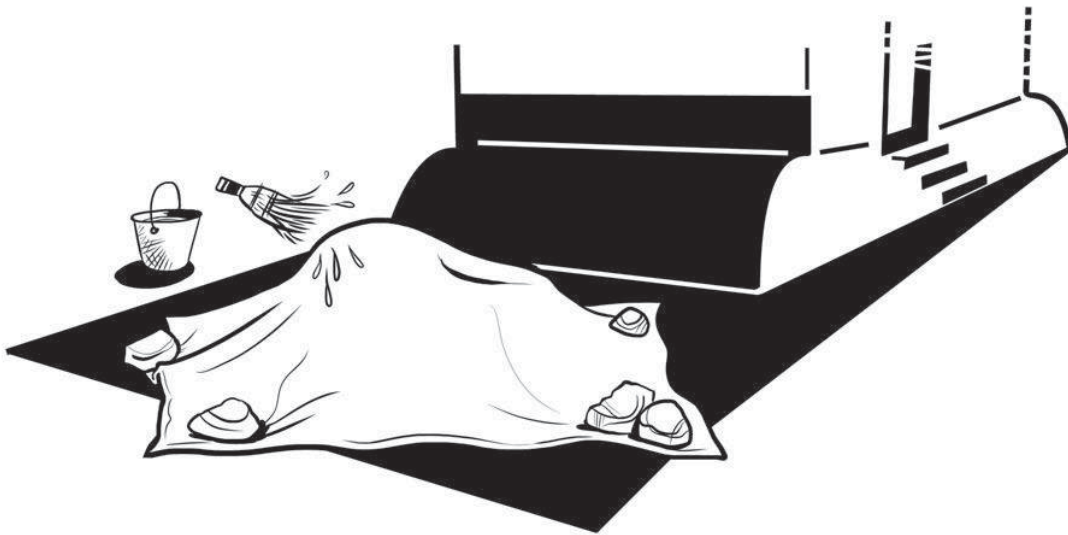
Fig 96 - Storage and Protection of Mixes
