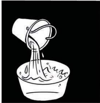
Fig 5: Always add Quicklime to Water, not water to Quicklime
