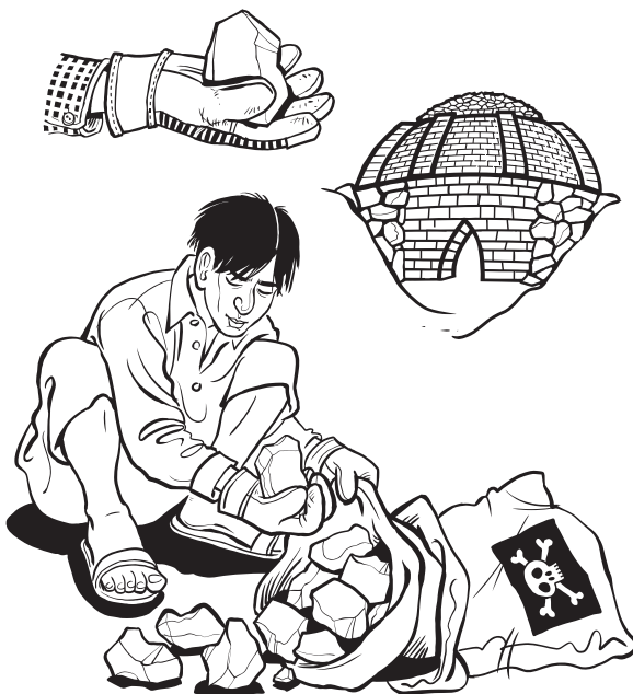
14a 3) Bagging quicklime into watertight and airtight bags
