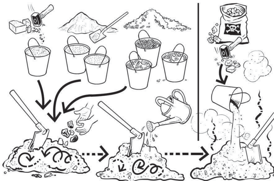
Fig 71: Likely locally available materials for foundations in Southern Pakistan: Lime, Clay Soil and sand and aggregates or Lime, Pozzolan, Sand and aggregates
