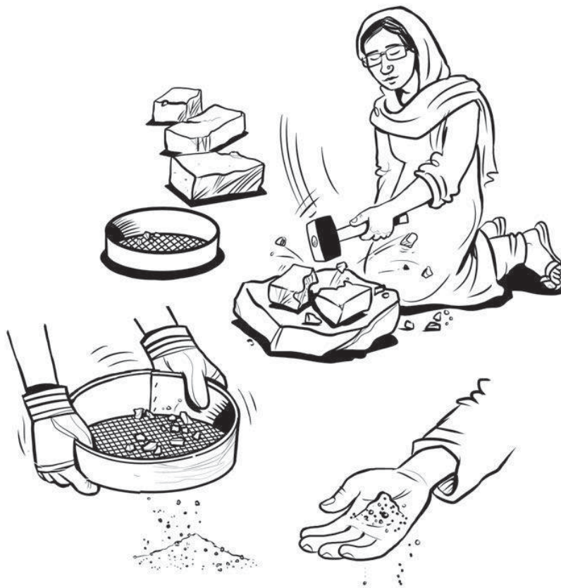
Fig 47b: The finer the pozzolan is ground, the more reactive it will be
