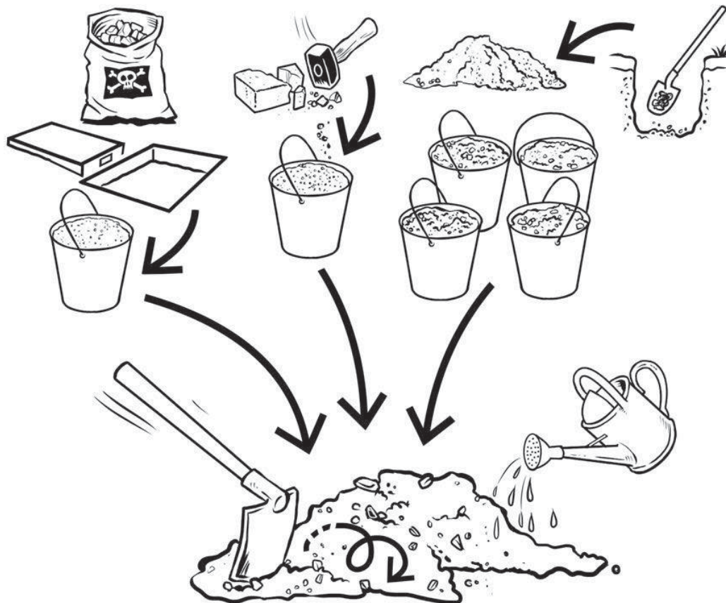
Fig 101: Trial render mixes with Lime Putty, Sand and Pozzolan (subject to testing). Try adding cow dung and fibre.
