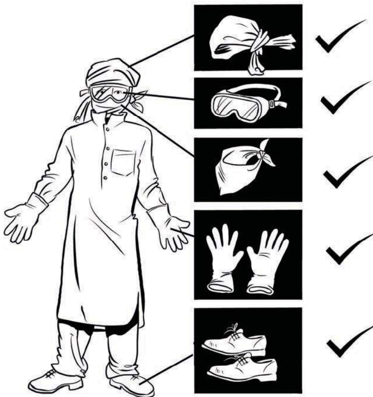
Fig 8: Wear Protective Clothing when working with Lime
