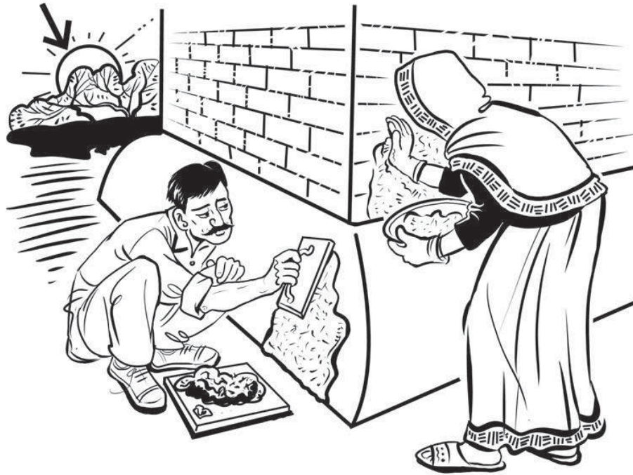
Fig 97: Apply render firmly to wetted background - if by hand, use gloves
