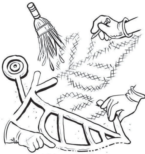
Fig 105: Raised Decoration: Scratch key the render and moisten before applying raised decoration
