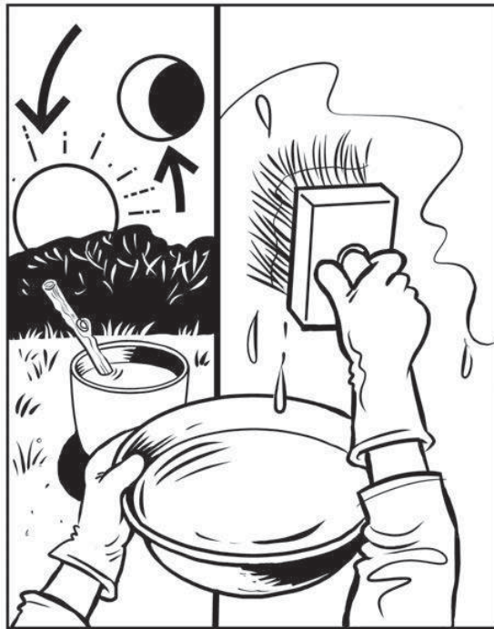
Fig 110: Applying next coat of Limewash: Leave 24 Hours before. Applying Subsequent Coats of Limewash
