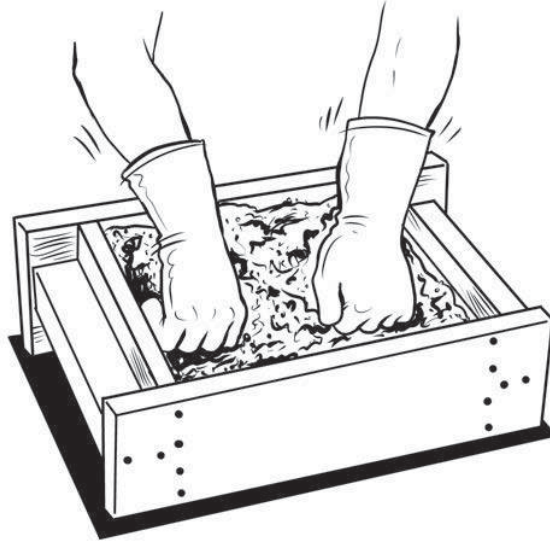
Fig 79 - Filling & Compacting the block mould
