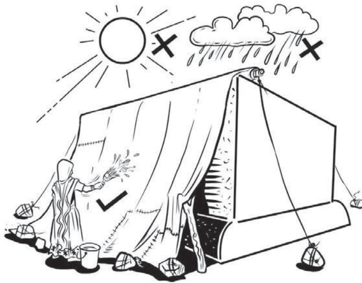
Fig 94b - Providing Shade for all lime stabilised work
