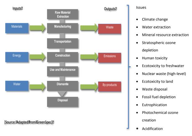
Figure 7: LCA assessment process including issues the methodology can address
