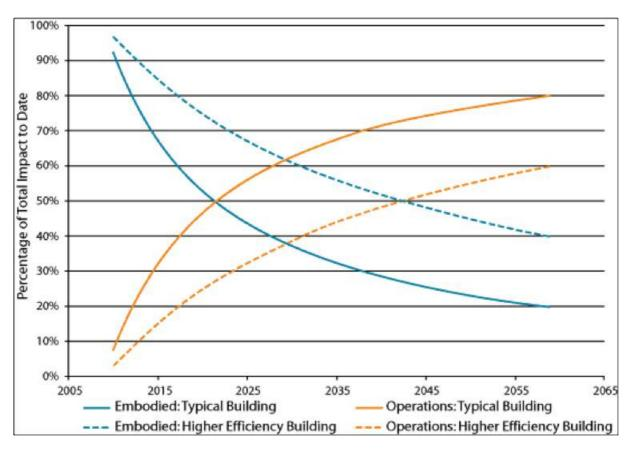
Figure 9: Embodied carbon and operational carbon in a typical building vs. a higher efficiency building
