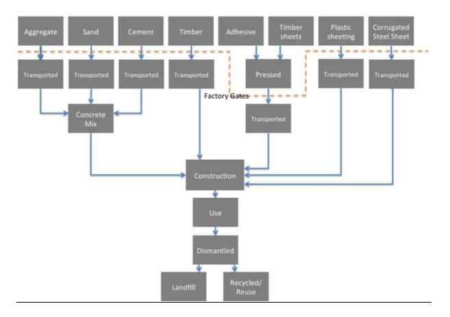
Figure 13: Temporary housing process tree
