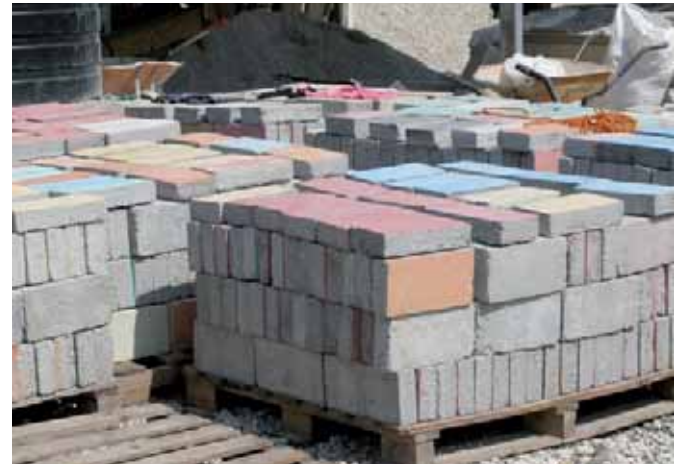
Paving blocks made out of crushed cement bricks, produced after the Haiti earthquake by IFRC's Integrated Neighbourhood Programme
