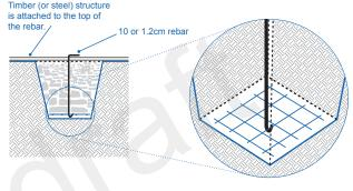
Step 1: dig holes - the size and number will depend on the design of the shelter
