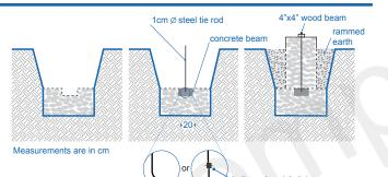
Step 1: dig a 60cm wide trench where the walls are to be constructed. Build up a stone or masonry footing with a channel for a concrete
