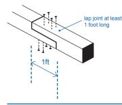
Or with a long lap joint - use a minimum of two nails or proper wood-to wood ioints and pre-drill all the timber before nailing to avoid splitting
