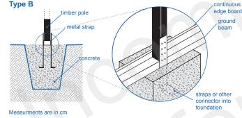
59. When using strip foundations or a stone base, a continuous ground beam (called a plinth beam) should be used to evenly spread the load of the structure onto the foundations. This is shown in diagram XX (adapted from ERRA/UN-Habitat, 2006).
