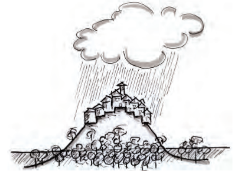
Construction on the highest level ground - advisable
