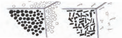
Aggregates with good shape and compacting (left) and bad shape and compacting (right)
