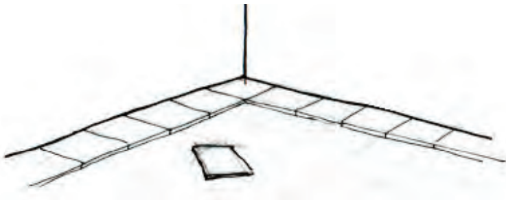
Tiles placing - starting from the corners
