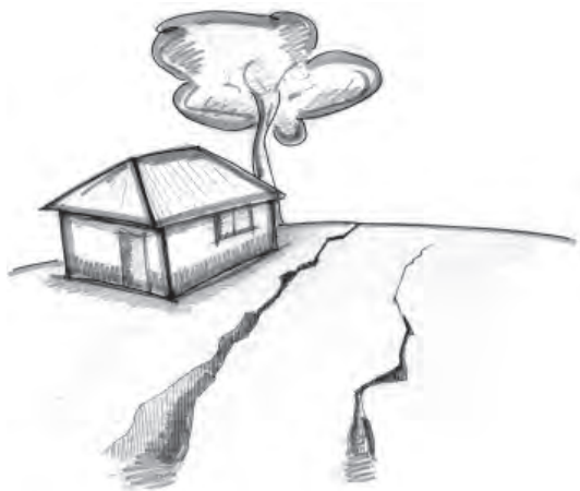
Presence of fault lines and trees - advisable to build as far away to these phenomena as possible
