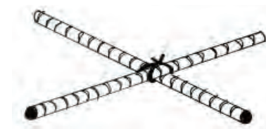
Tying two bars together
