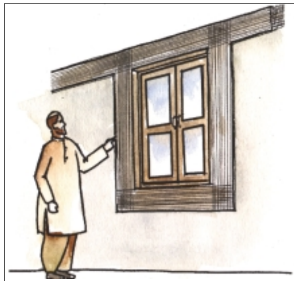
Installing WWM around window opening
