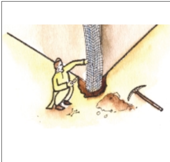
Anchoring vertical belt 300 mm below plinth level
