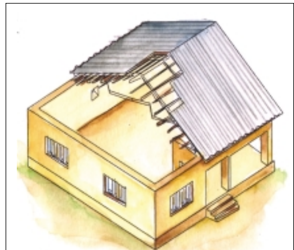
Collapse of a portion of roof
