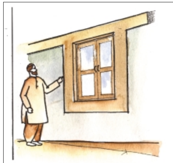
Completed encasement belt around window
