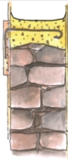
Seismic belt shear connector
