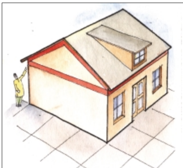
Belt reinforcement at opening
