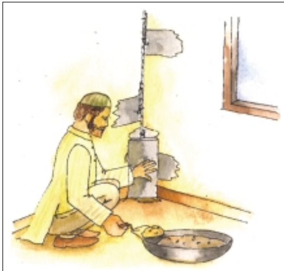
Encasing vertical rod in concrete
