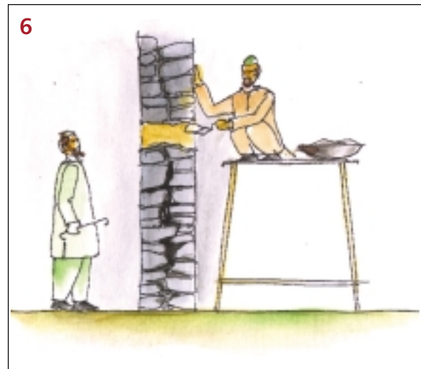
6 Placing concrete and rebar in the hole
