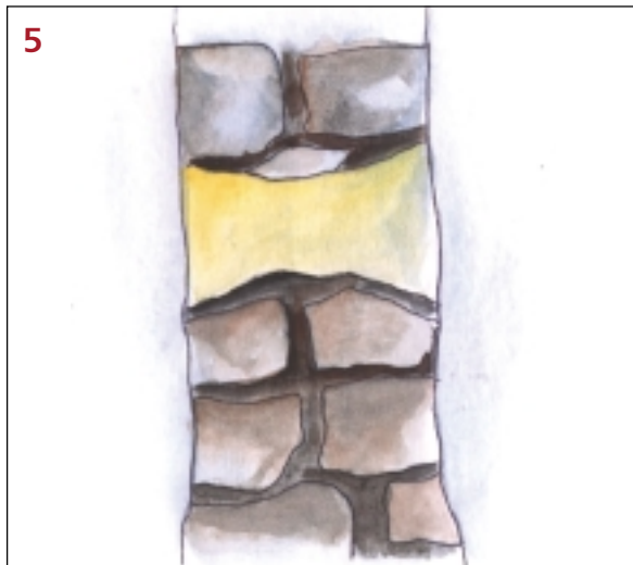
5 Making dumb-bell shaped hole through wall
