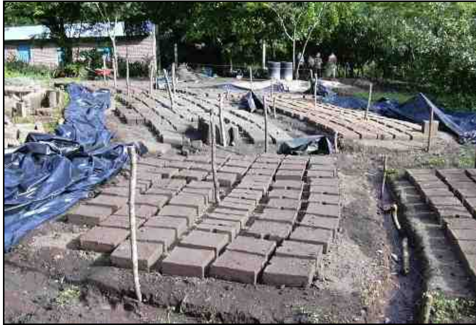
Figure 3. Drying bricks (Note: drainage ditches and plastic covers)
