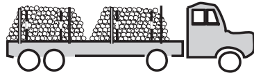
DO NOT stack timber across a truck – it is likely to fall
