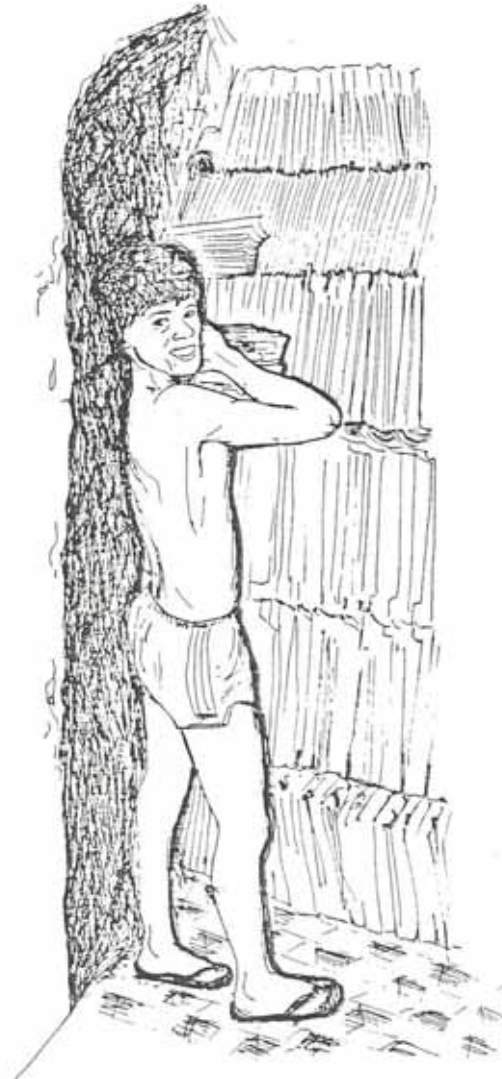
Figure 30: Stacking the tiles in the kiln.
