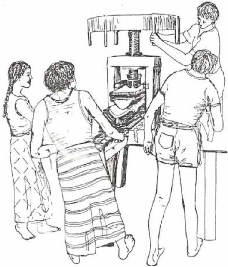
Figure 24: Pulling the lower die from the press.
