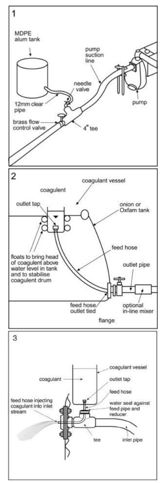
the Tee and into the incoming water flow and coagulant introduced at a constant rate.
