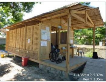
The iron sheet roof covers the whole shelter. It is made of a double sloping roof gradient 3/10 which limits wind intrusion.
