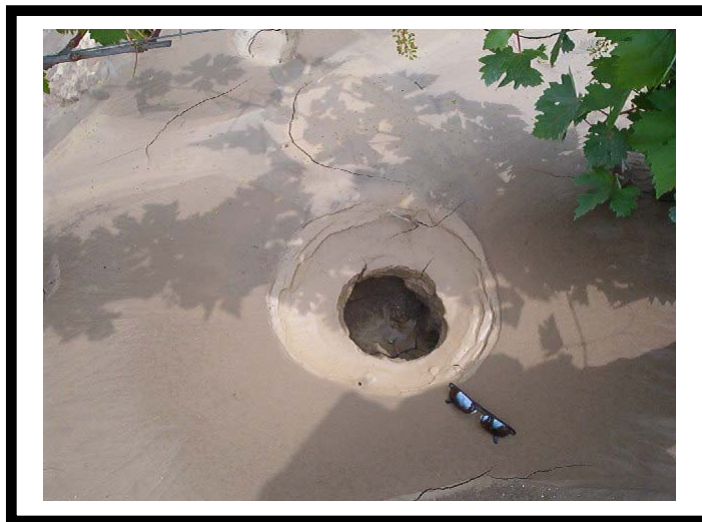
Photo 2: Shows liquefaction phenomenon during the 2003 Boumerdes (Algeria) earthquake.
