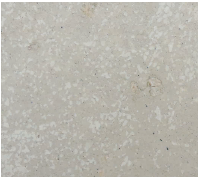
Sample 10 (4% Cement) After 30 Days Subjected To External Conditions
