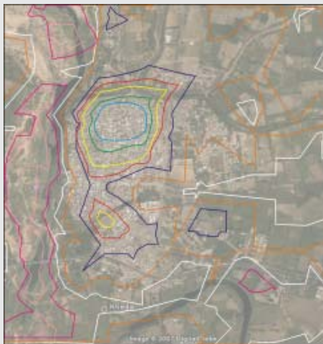
Figure: This map of Kheda is based on maps from Google Earth. The scale of the map is 1:16000 (1 cm = 160 m = 525 ft). The purpose of this map is to show which areas in the city are in danger during high water. Though the map is not 100% accurate, it can give a good indication of the areas where the water will go in case of heavy rainfall or floods. The floods of 2006 confirm this; one low-lying slum area became one of the first areas to be flooded, almost exactly according the elevation line of 24 meters. AIDMI has been active in the slum area as well as in a slum area on the north side of Kheda City.
