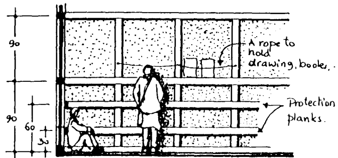
Prevent damage by students to ekra walls.
