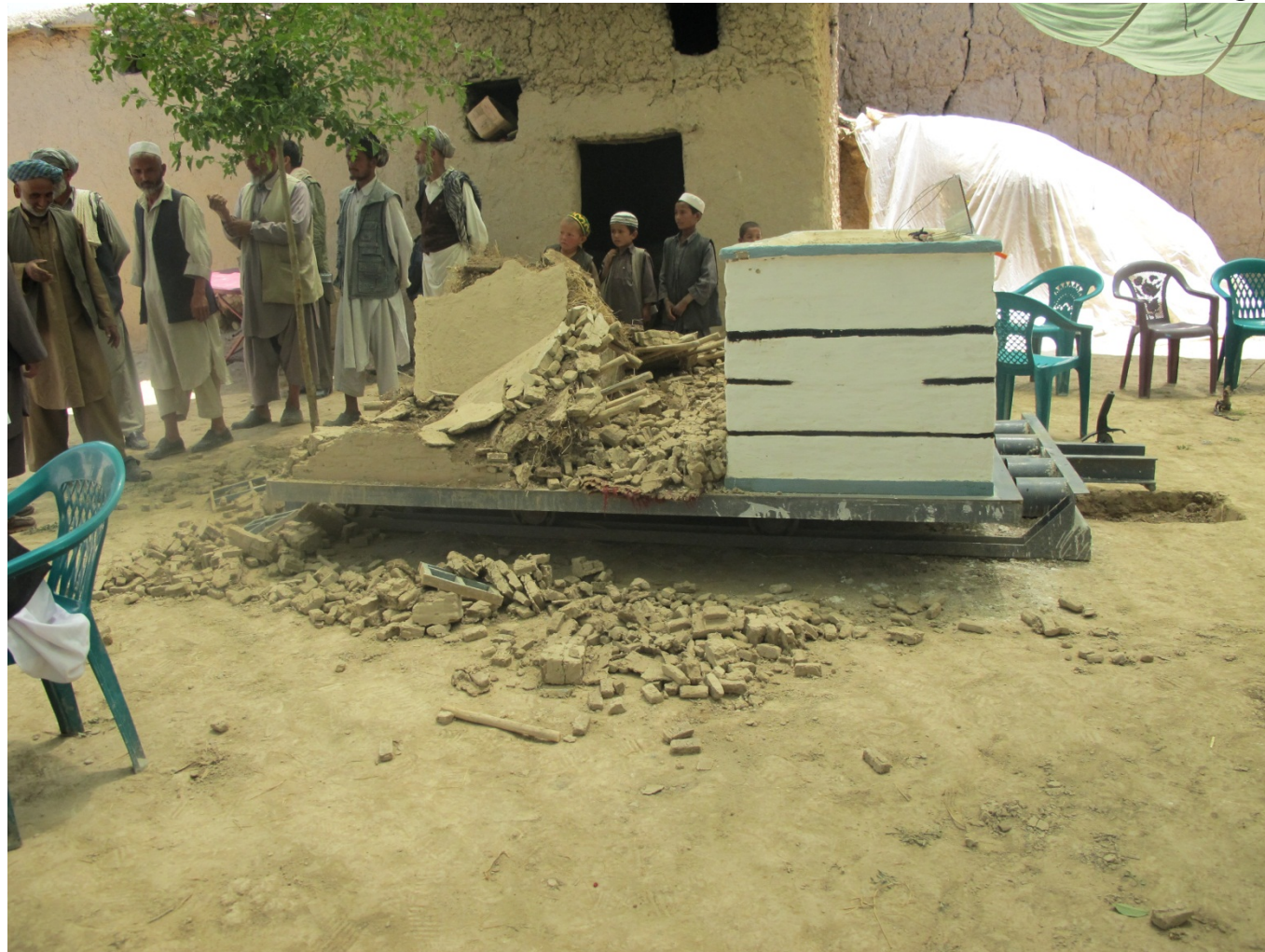
The traditional structure collapses while the improved unit allows time for escape.
