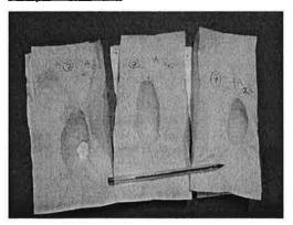
Figure 16(b): Example of Burned Sample
