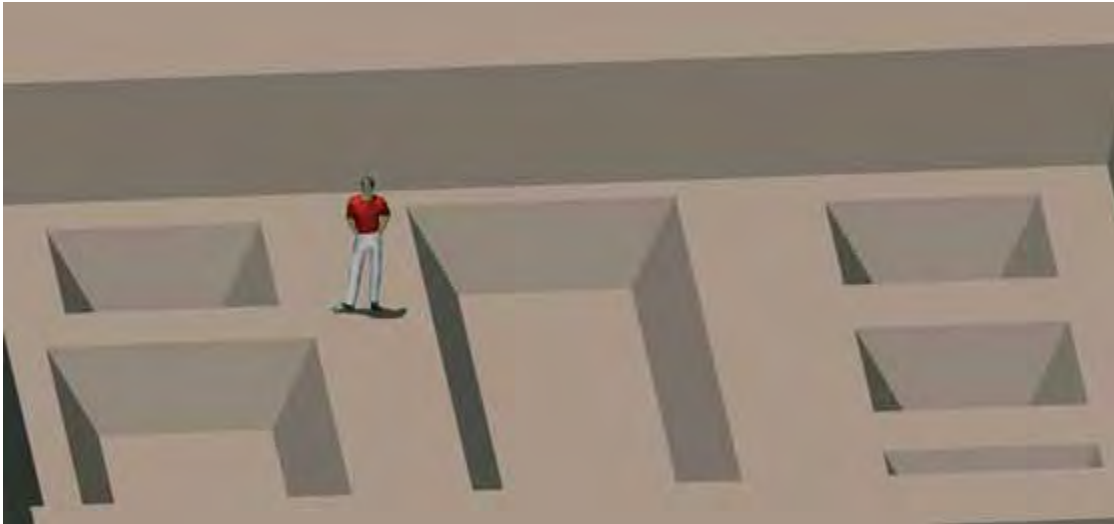
Excavation for foundation with terraces
