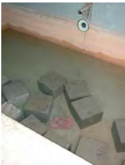
Curing of testing blocks
