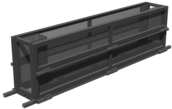
18 | Mould designed to make the element
