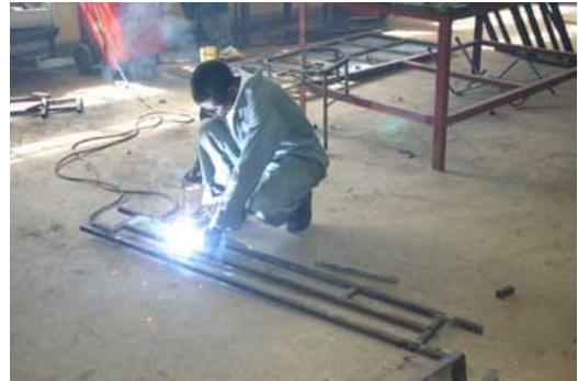
33 | Manufacturing the moulds
