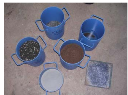
24 | Materials for the concrete mix
