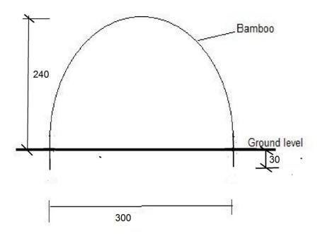
• Reinforce the arch by placing bamboo at the side. Use cable tie to fix the bamboo slices
