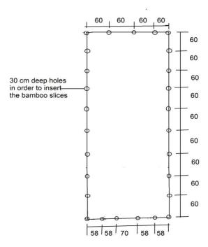
• Place the cut bamboo in the holes as shown in the figure below. The bamboo will form an arch shape due to its flexible nature
