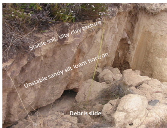
Figure 7: Alternation of stable pedogenesis phases and unstable phases of regressive erosion
