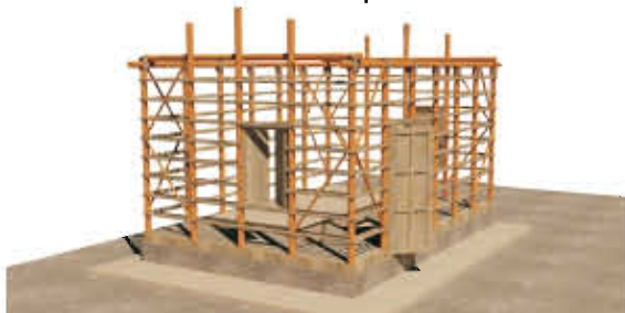
Bracing & horizontal plates
