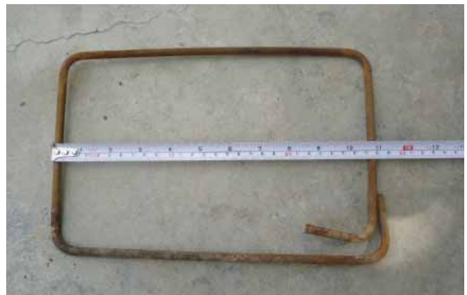
Rebar Hooks, ends are not bent inside.
