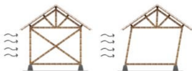
EFFECT OF WINDLOAD ON BUILDINGS WITH AND WITHOUT BRACING
