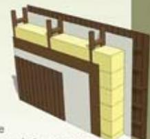
Bamboo frame construction with straw bales as an insulation inbetween.
