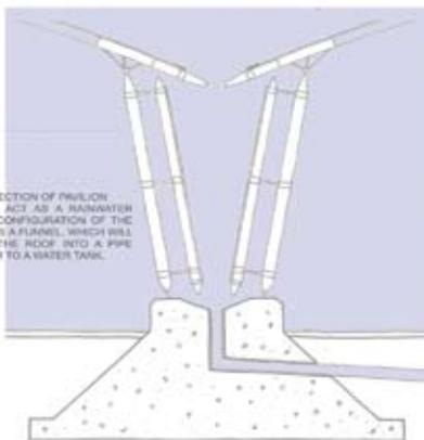
THE ENTIRE STRUCTURE UTILISES A COMBINATION OF MATERIALS, PREDOMINATELY BAMBOO WITH STAINLESS STEEL CONNECTION DETAILS AND CONCRETE FOUNDATIONS. THE ROOF SKIN WILL BE AN IMPERMEABLE CLOTH MATERIAL SUCH AS SAIL CLOTH, THIS WILL ALLOW TRANSLUCENT LIGHT THROUGH THE STRUCTURE, CREATING A SHADOW PATTERN OF THE RAFTERS ON THE FLOOR.
