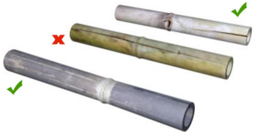
MINOR SPLITTING, MAJOR SPLITTING AND END SPLITTING
