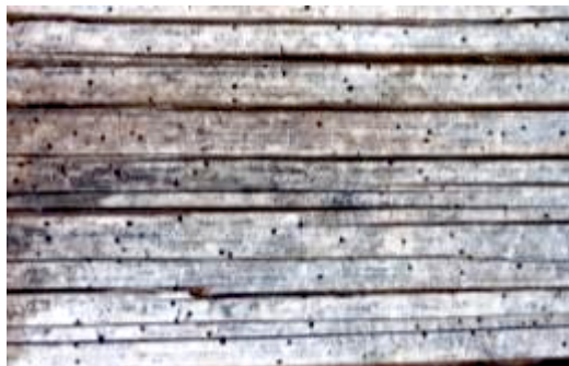
PINHOLE BORER ATTACK ON AGING BAMBOO SHEETING
