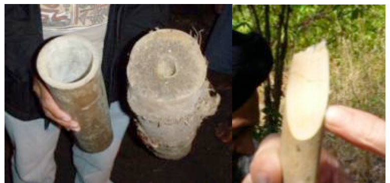
EXAMPLES OF SPECIES DIVERSITY: THIN-WALLED BAMBOO SUITABLE FOR RAFTERS, THICK-WALLED SUITED TO POLES AND SOLID BAMBOO USED FOR HAMMER HANDLES
