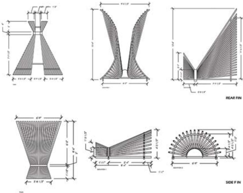
These fins are constructed with structural bamboo pieces of 2 and 3" diameter. The pieces are connected to main members at steel joints or with steel bolts. The entire structure is on wheels. The model is made from cocoyea sticks, which are the centre trips of coconut leaves.
