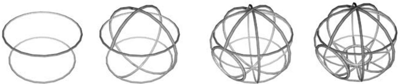
Coconut's concept aims to combine design and structure in a perfect balance. In order to achieve this result, coco features an innovative method of construction which employs only bamboo curved poles. The greater poles are curved while they are still growing, while the thinner ones are bended relying only on the natural flexible power of bamboo. Like a basket, in coco every element plays a key role making harder the whole structure at every
