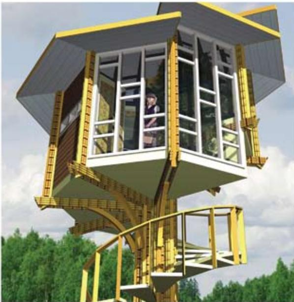
Attic\_3 is a multifunctional bio-ecological living/housing/work unit. Its structure is adjustable to its environment and the user's requirements. The structure is applicable in rural, as well as in urban environments. The core of the building is a tree or a lamppost, surrounded by a stable structure of bamboo pillars on which eight floor boards are attached that can differ in height. Using these parts, rooms of various sizes and levels can be created. The stairs that lead to the residence
