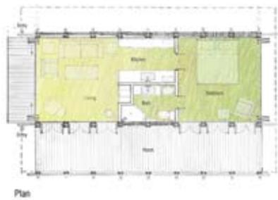
The elevated resort house offers a simple yet effective design response to the connection of the structure to any surrounding landscape. The small house contains a living area and a bedroom area connected by a bath and kitchenette. A series of doors merges interior and exterior space by opening up to a large covered porch that spans the entire length of the structure. In addition to the porch, both ends of the house can be completely opened to the surroundings with a system of folding shutters.
