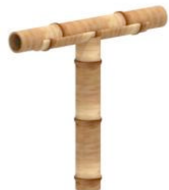
DETAIL: Top plate with fish-plate where posts intersect support
