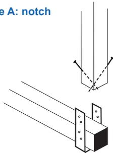
Timber beams and ring beams connections should be secured with a notch of 1 inch in the corners.
