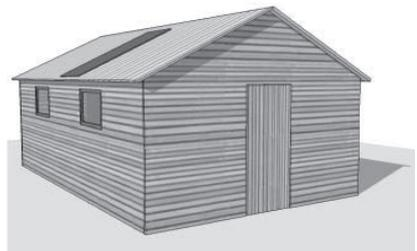
*Semi-permanent house with wooden panels as wall and corrugated iron sheeting on the roof. The house is fitted with a solar panel for electricity.*
