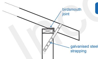
Galvanised iron strapping is used to reinforce diagonal timber braces, and should be carefully nailed over all connections
