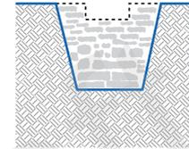
**Step 2:** assemble formwork to 30cm above the ground and as wide as the wall. Tie bars should be attached to the formwork reinforcement with wire. The bottom of the tie bar should be at least 25mm away from the rubble.
