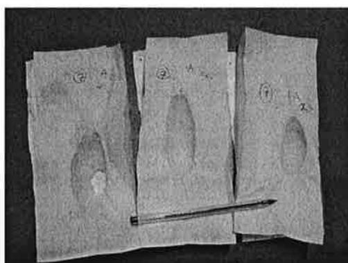
Figure 16(b): Example of Burned Sample
