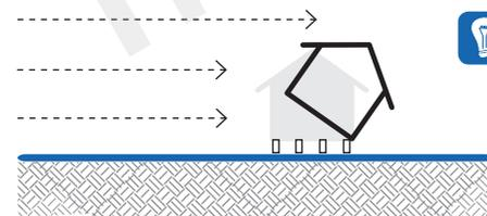
Foundations should be appropriately dimensioned to make shelters withstand uplift forces in strong winds.
