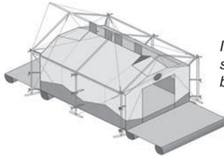
*Integral flue plate for stove is held in place by cable tensioners*
