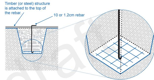
**Step 1:** dig holes - the size and number will depend on the design of the shelter
